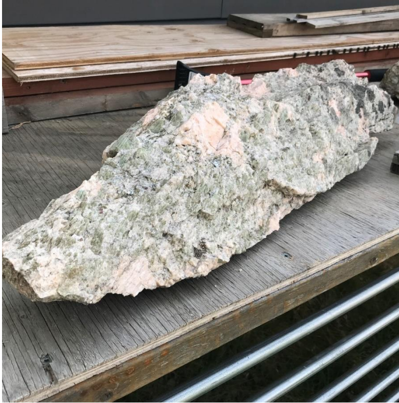
Figure 6-4: An example of part of a pegmatite dike with spodumene (green) and potassium feldspar (pink) megacrysts
