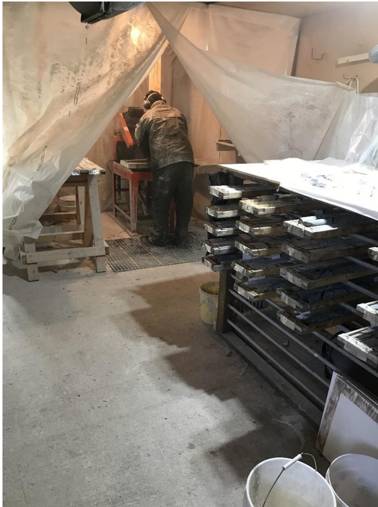
Figure 8-2: The core cutting facilities using the diamond core saw. Core racks outside of the cutting area hold core boxes that are awaiting cutting.
