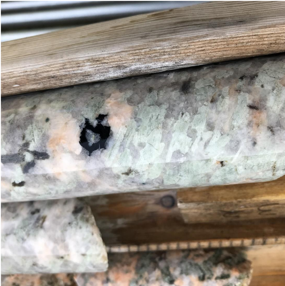
Figure 6-5: Piece of drill core showing the presence of spodumene (green), potassium feldspar (pink), biotite (black) and tourmaline (light to dark grey)
