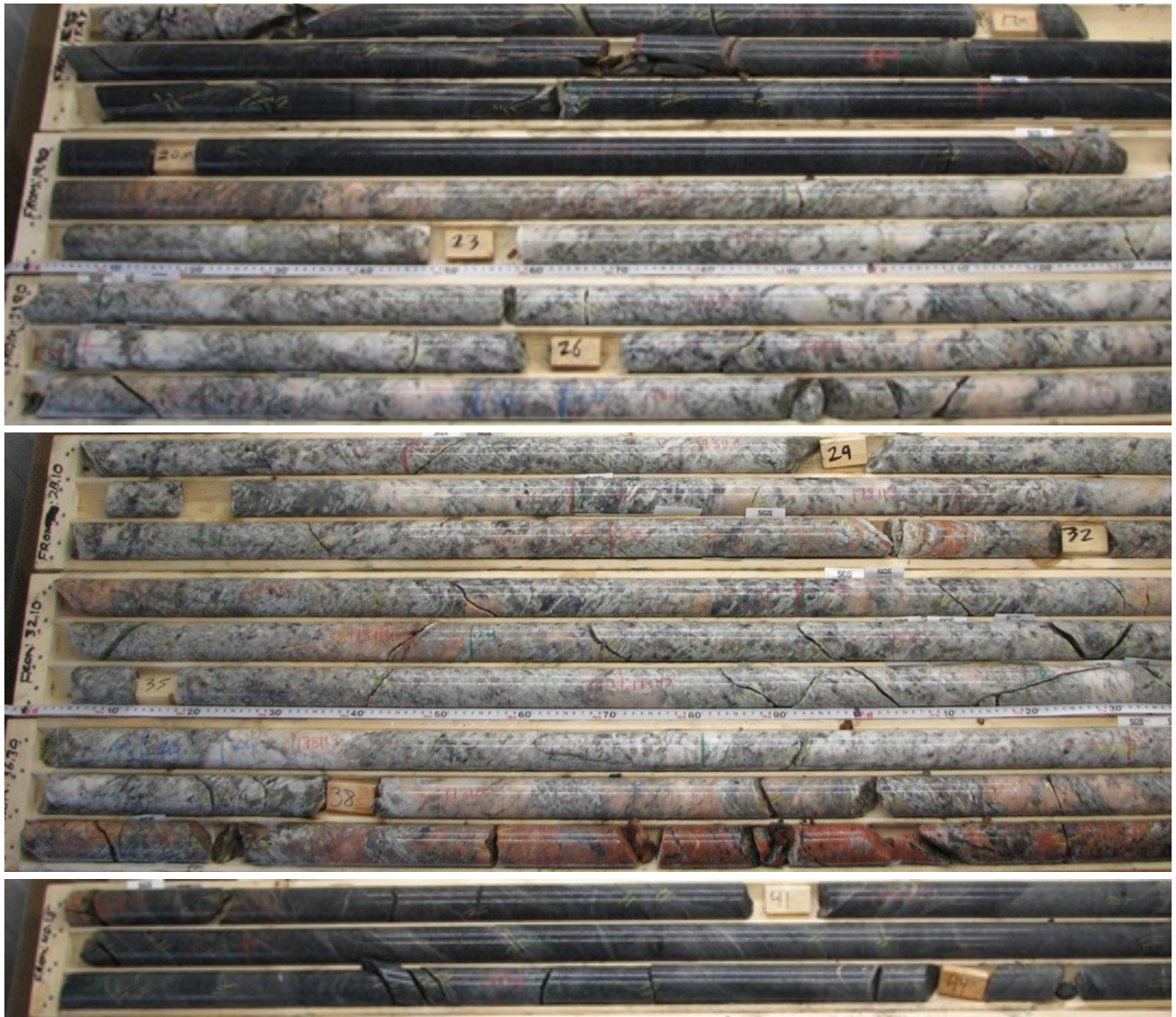
Photo 2.0 - Spodumene Pegmatite from TBL-025 have an intersection of 19.8 meters core length (~ 14.0 meters true width) from 21.0 to 40.8 meters.
