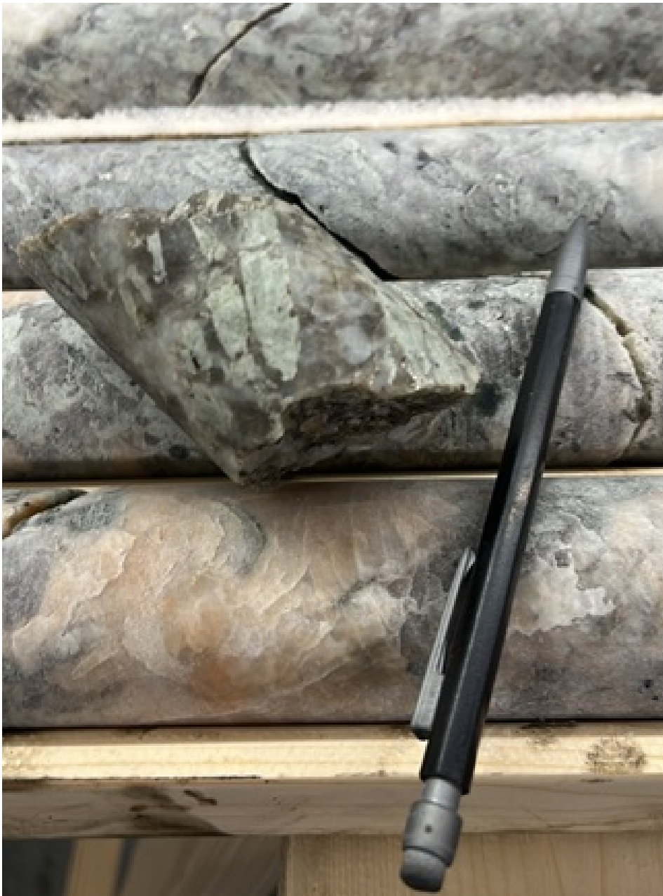
Photo 1.0 Core sample from TBL-025 containing 20 to 25% spodumene. Intersection is from 21.0 to 40.8 meters.
